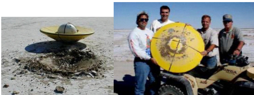
EEV development model dropped tested at UTTR, reached terminal velocity
