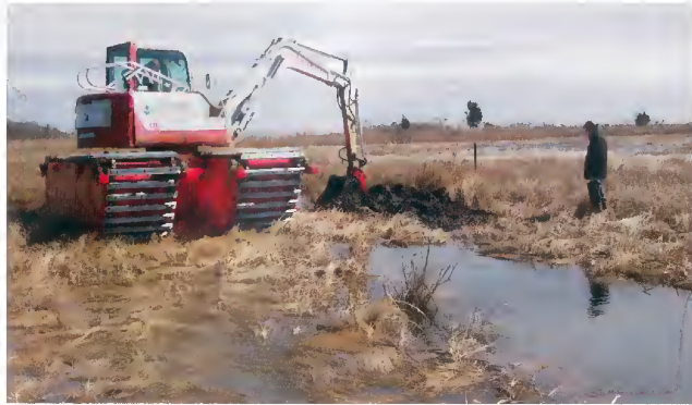
Figure 5: To fill a ditch, excavators must find a source of fresh peat. So peat is excavated from intact high marsh. In the process, new ponds and ditches are dug. Areas scouted for peat removal are those that are wet with puddles or small pannes. From Figure 21, page 91 of the Memoirs (image credit: National Park Service)
