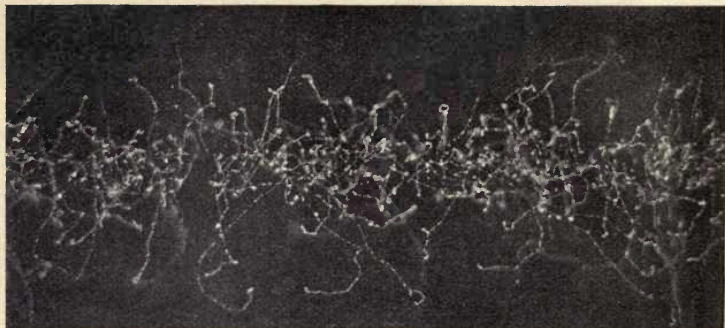
FIG. 1.—Photograph obtained by C. T. R. Wilson of the path of a beam of X rays in supersaturated air. The beam of rays, some 2 mm. in diameter, was sent through the moist air (from left to right in the figure) immediately after the expansion which produced the supersaturation (see p. 149). The axis of the camera was horizontal, and the magnification of the photograph is about 2\frac{1}{2} times.
