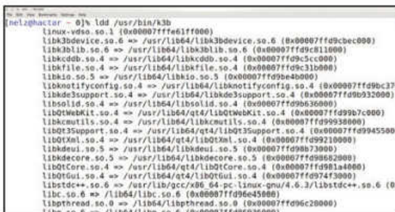
» Shared libraries enable a more efficient system, by sharing code between applications. Here are just some of the libraries the K3b disc burner links to.
