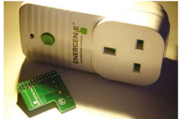
» The receiver in the Energenie unit houses a relay to switch the mains power on and off.
