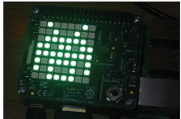
➤ The Sense HAT fits neatly on the Pi and leaves plenty of space to attach the new Pi display and camera.
