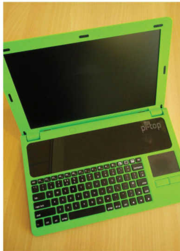
» Pi-Top isn't quite your typical laptop, and under the lid it's all Raspberry Pi powered.
